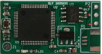
2. Connect ELV Emulator to car (original ELV must be connected too). +12V, GND and TX (TX it is LIN) 3. Switch Ignition ON , LED on EMU should Blink (sometimes can blink few times) , and don't switch OFF ignition <a>!!!!</a>
